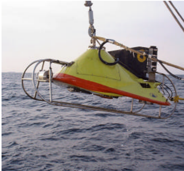
Figure 6. The Greene Bomber is a V-fin towed body equipped with a dual frequency (120 and 420 kHz) down-looking echosounding system and suite of environmental sensors.
