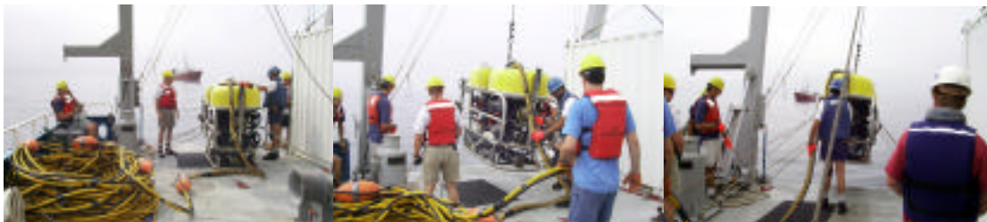
Figure 10. Launching the Kraken ROV from the R/V Connecticut in Cape Cod Bay on the morning of Aug 12, 1999. The F/V Isabel S can be seen in the background.
